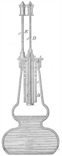
cover. The graphite is in the form of a cylinder and is secured as described further on. Upon the cover are the two electrodes, D and E, consisting of rods of brass at the upper extremities of which are spring clamps which hold the spiral of platinum wire. One electrode, D, is attached directly to the cover, the other, E, carries the graphite cylinder, and is isolated at its point of contact with the cover by a rubber en velone.
