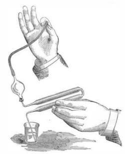
by touching the point, a, with a little roll of filter paper. Supposing, however, that in so doing too much liquid is abstracted, capillary force will redress the fault, if point, a, be touched with a drop of the liquid under examination; for this gentle force acts instantly through the whole mass of the liquid, causing it to move forward again to or beyond the mark.
