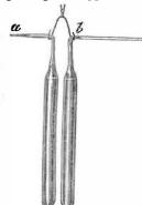
point, however, which I wish to notice more partioularly (for reasons explained below) is the different caliber of the two capillary tubes. The shorter one is a good deal narrower (at least towards the end) than the longer one, the inner diameter of which is about .02 of an inch. The horizontal part of this wider tube is marked near the bend with a delicate line, b. This line and the extremity of the opposite capillary tube, a, are the marks which limit the volume of the liquid to be weighed.
