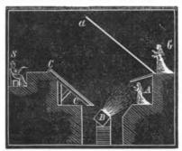
tator in front of the stage, as at 8, the figure appears to proceed from a point G, behind the glass. Really, the figure would appear to be back of the glass as far as the image formed in the mirror was in front of it, and thus the spectator does not perceive the plate glass.
