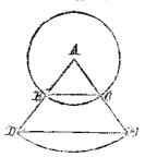
lever can be found by a simple proportion. Example Diameter of steam chest = 6 inches. Travel of valve = 5 inches. Throw of eccentric = 11 inches. Angle B A C=  $5 \times 360 + 188496 = 95^{\circ}30'$  nearly. Chord B C =  $6 \times 0672$  =  $4\cdot032$  inches. Lever A E =  $3 \times 11 \div 4\cdot032 = 8\cdot18$
