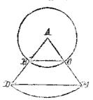
lever can be found by a simple proportion. Example Diameter of steam chest = 6 inches. Travel of valve = 5inches. Throw of eccentric = 11 inches. Angle B A C=  $5 \times 360 + 18.8496 = 95^{\circ}30'$  nearly. Chord B C =  $6 \times 0.672$  = 4.032 inches. Lever A E =  $3 \times 11 + 4.032 = 8.18$
