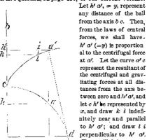
nitely near and parallel to h' a'; and draw l i perpendicular to h'  $\alpha'$ . Then will l i represent d x and a' i' will represent d y. Now because x may vary
