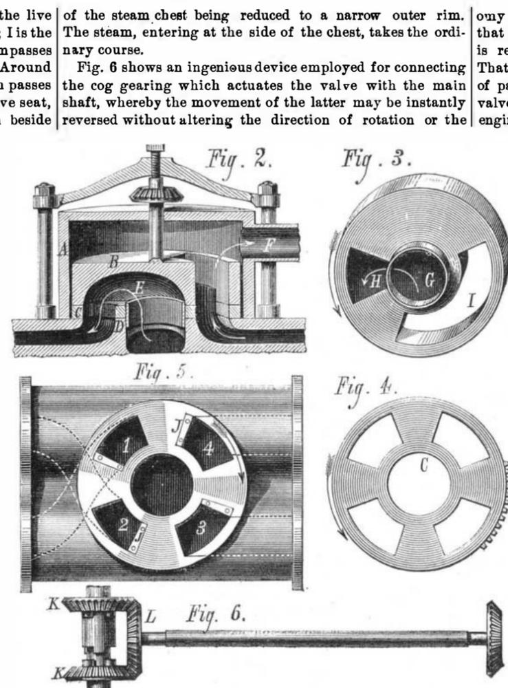
of the steam chest being reduced to a narrow outer rim. The steam, entering at the side of the chest, takes the ordinary course. Fig. 6 shows an ingenious device employed for connecting the cog wheel which actuates the valve with the main shaft, whereby the movement of the latter may be instantly reversed without altering the direction of rotation or the
