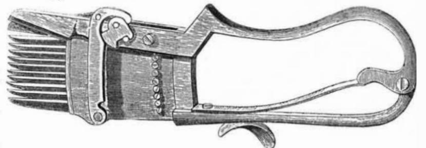
work than the most skillful shearer with the old fashioned shears, and without danger of cutting the flesh. The handle of the knife is arranged with a spring, and the blade, by pressing the former, is caused to travel across the sharp teeth, which are first imbedded in the wool. The movement resembles that of the ordinary scissors blade. When the knife returns, it raises itself clear of the wool, allowing the same to escape uninjured by scraping.
