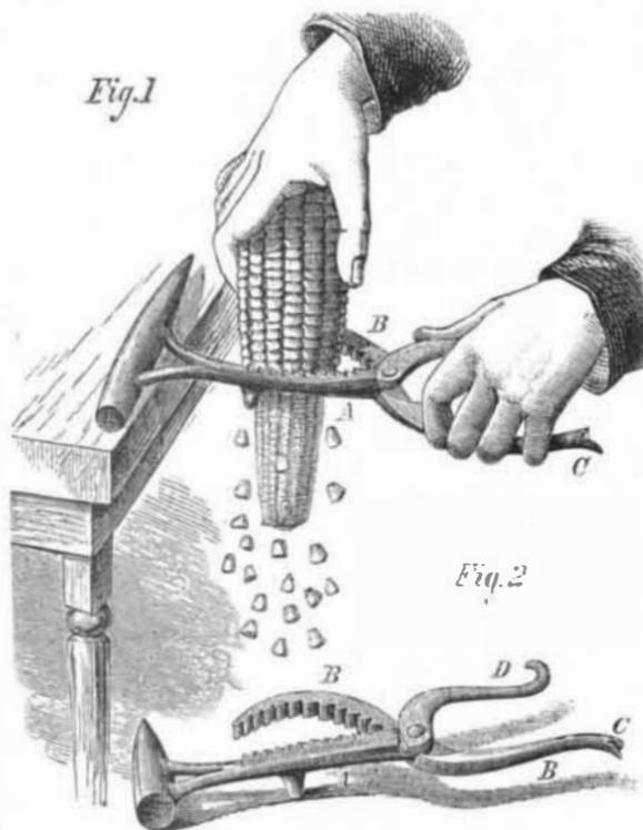
in the single instrument represented in our engraving, the construction of which amounts to simply three pieces of metal fastened together by a single rivet. Mr. Anthony Iske, of Lancaster, Pa., is the inventor, and he clearly deserves credit for no small amount of mechanical ingenuity.
