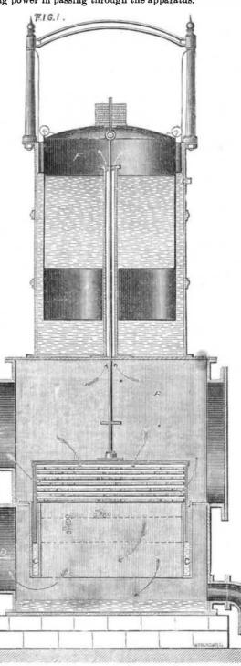
A is the condensing apparatus, properly so called; B is the chamber in which the apparatus moves; C is the inlet for gas; D is the outlet for gas after passing the condensing apparatus; E is the outlet pipe for condensed products, terminated by a siphon; F is the regulator, by means of which the number of perforated plates in use is varied according to the quantity of gas to be purified; and G is the water space into which the apparatus dips.—Journal of Gas Lighting.
