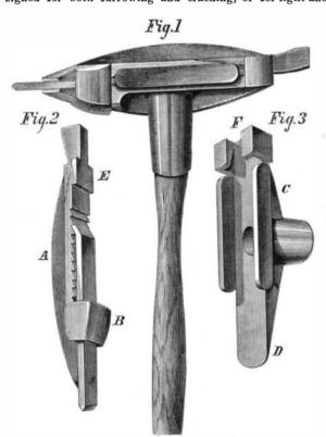
heavy stone dressing. The principal advantages are the firmness with which the blades are held, the manner of letting the same down, to compensate for wear, and also the facility with which they may be changed. The latter is an important feature, as it is often necessary to remove blades for sharpening as many as one or two hundred times in dressing a mill or a run of stones. Two sizes of the implement are made, one for furrowing and the other for cracking.
