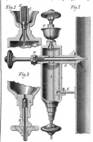
above the boat and in condition to be fed through the open ings. The mere action of the valves, therefore, when steam is shut off from the cylinder, it is claimed, is sufficient to bring the oil away, so that the lubricant is supplied just when the facings become dry and cutting begins.
