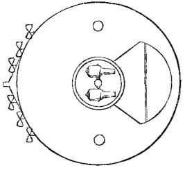
At the center of the ship is a turret, 29 feet 6 inches in diameter and ? feet high, containing two 11 tun steel guns (probably eight inch bores), breech loading and mounted en barbette. The turret has a hollow axis which serves as an ammunition scuttle, and on which pivot the supports of the guns, so that the latter can be pointed over an angle of from 30° to 35° with the fore and aft direction of the ship. The rest of the armament consists of torpedo arrangements.
