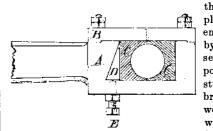
the stub end; B, plate or cap fastened at each end by a stud, an offset fitting a corresponding one upon stub end A; C C are brasses; D is a steel wedge to take up wear of boxes or brass es, adjusted
