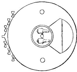
At the center of the ship is a turret, 29 feet 6 inches in diameter and ? feet high, containing two 11 tun steel guns (probably eight inch bores), breech loading and mounted en barbette. The turret has a hollow axis which serves as an ammunition scuttle, and on which pivot the supports of the guns, so that the latter can be pointed over an angle of from 30° to 35° with the fore and aft direction of the ship. The rest of the armament consists of torpedo arrangements.
