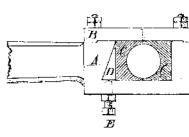
the stub end; B, plate or cap fastened at each end by a stud, an offset fitting a corresponding one upon stub end A;  $C \subset are$ brasses; D is a steel wedge to take up wear of boxes or brasses, adjusted
