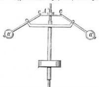
center of ball, a, to c, is 39 inches: How much pres sure will be exerted upon the sliding sleeve (A) by both balls? [This is a simple and interesting problem, requiring the application of the principles of centrifugal force and of the lever for its solution. We believe that some of our readers take an interest in such matters. and wepreferto leave to them the solution of the question.-Ens.]
