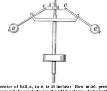
sure will be exerted upon the sliding sleeve (A) by both balls? [This is a simple and interesting problem, requiring the application of the principles of centrifugal force and of the lever for its solution. We believe that some of our readers take an interest in such matters. and weprefer to leave to them the solution of the question.-EDs.]
