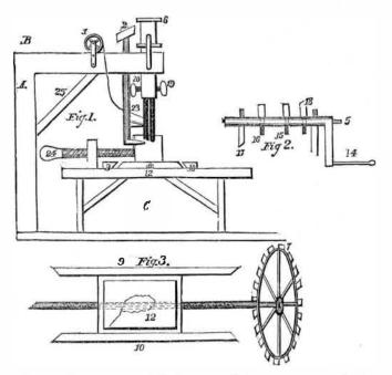
the stitch and keeps it tight till the needle has brought another stitch through the last taken; and so it goes on alternately until the whole article is completely stitched. 3 is the awl that makes the holes for the needle to pass through, 5 is a spindle that goes through the poppet at 6; while by turning the spindle at 5, the awl and needle is worked by the cogs 15 and 16, which are in the spindle at 5; and the motion of this spindle gives motion to the prongs 26 and 27, which
