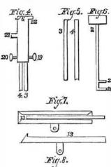
are in the spindle at 2. 14 is a cogthat gives mogives motion to a slide at 12 which moves along the grooves at 9 and 10 by means of a screw that is fixed in the wheel, to which slide the article is fixed for stitching. The prong 26 goes into a hole at the slide 13 and gives motion to it "which draws the thread on the under side of the article and ho'ds it tight till the next stitch is taken, and so on till it is done. 22 in Fig. 6 is a shoulder
