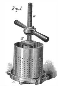
A is the base of the apparatus, having radial corrugations raised upon its surface, the channels between which lead the rpressed liquid to the spout shown. short conical projection, over which fits the lower portion of an inner perforated tube, A. The latter is connected with
