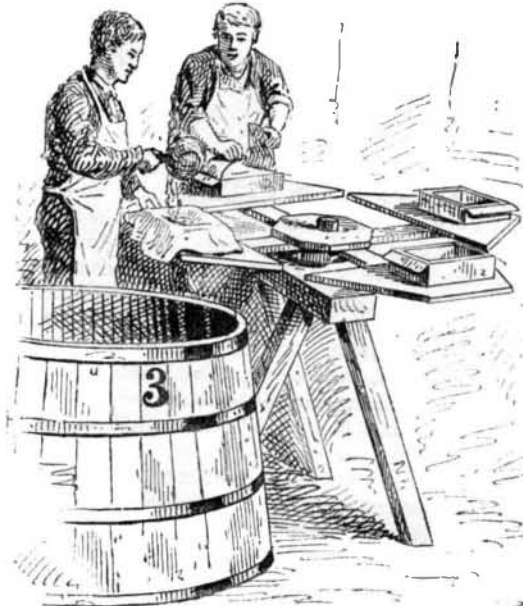
MANUFACTURE OF ARTIFICIAL BUTTER.—FILLING THE BAGS FOR THE PRESS.
