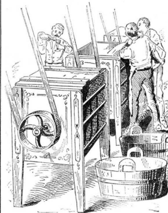
MANUFACTURE OF ARTIFICIAL BUTTER.—CHURNING THE OLEIN WITH MILK.
