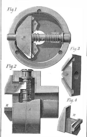
The shaft, C, is directly in line with and above the slot in which moves the jaw, B; and from the section, Fig. 2, it will kinds of fuel of this description. It required 46 minutes to of least pitch on the shaft; so that, as said shaft is rotated, nearly finished. It is about 3,000 feet long.
