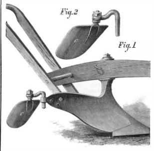
share. A bed of friable soil is thus prepared, excellently suitable for the germination of the seed. To cover the latter. it is simply necessary to use the plow without the attachment, the ground being thrown up and over the potatoes by the moldboard in the ordinary way.
