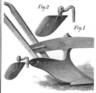
share. A bed of friable soil is thus prepared, excellently suitable for the germination of the seed. To cover the lat. ter. it is simply necessary to use the plow without the attachment, the ground being thrown up and over the potatoes by the moldboard in the ordinary way.
