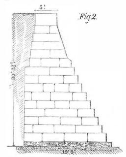
on a bed of concrete and riprap. The hight is 30 feet  $3\frac{1}{4}$ inches. Behind this wall, however, is merely earth thrown in and not packed or rammed down,-a precaution, in fact, not as yet taken, because no craft larger than a ship's launch was expected to come near the work. The consequence was that the loose soil yielded, while the ship escaped with no other injury than some scratches and a lump of granite imbedded in her bow.
