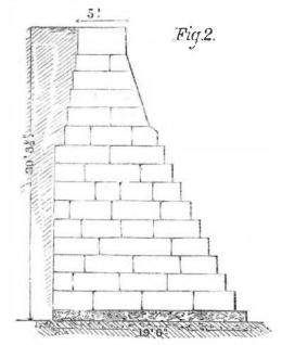
on a bed of concrete and riprap. The hight is 30 feet 31 inches. Behind this wall, however, is merely earth thrown in and not packed or rammed down,—a precaution, in fact, not as yet taken, because no craft larger than a ship's launch was expected to come near the work. The consequence was that the loose soil yielded, while the ship escaped with no other injury than some scratches and a lump of granite imbedded in her bow.
