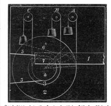
Scale 1¼ inch to the foot. 1, stick of timber 12 inches through. 2, circular saw 60 inches in diameter. 3, circu-lar saw 30 inches in diameter. 4, 24 inch pulley. 5, 5, driving beit. 6, pitch line drawn to ¼ the diameter of saw. 7, pitch line drawn to ¼ the diameter of saw.
