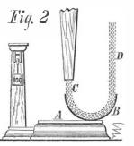
platform, B the curved plate, and C and D the falling and rising columns of water. The conditions, however, thus determined are modified through the motion of the point to which the power is applied. Thus, if a wheel could remain stationary and still transmit the impulse,
