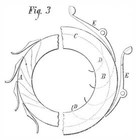
The inventor proceeds further to state that, in some well known turbines, the direction of the water must be deflected inward against this centrifugal tendency, a force augmented by the motion of the wheel. This deflection increases the action of the water against the point of the chute, but diminishes that in the inward direction, through
