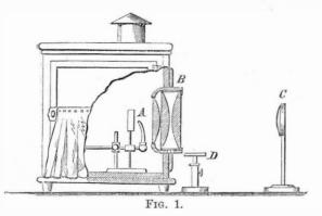
A magic lantern consists essentially of a box to inclose the source of light, say a lime light, as at A, a series of lenses called the condenser, whose office is first to collect the scattering 1ays, from A, that fall upon it and bring them into a common direction, and, secondly, to so converge or condense them as to make them all enter the object glass or object tive, C.
