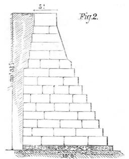
on a bed of concrete and riprap. The hight is 30 feet  $3\frac{1}{2}$  inches. Behind this wall, however, is merely earth thrown in and not packed or rammed down,—a precaution, in fact, not as yet taken, because no craft larger than a ship's launch was expected to come near the work. The consequence was that the loose soil yielded, while the ship escaped with no other injury than some scratches and a lump of granite imbedded in her bow.
