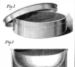
The advantages claimed are economy in the use of blacking, none being wasted by caking in sharp corners, ready removal or affixing of the cover, and the absence of rough or sharp edges which cut the brush. Patented July 11, 1871. For further particulars address the inventor, Mr. Dennis O'Leary, Hubbard, Trumbull county, Ohio.
