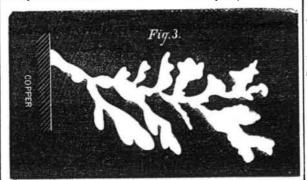
croscope. A stronger solution gives white crystals from the commencement, which frequently assume the appearance of fern leaves; the analogy between crystals and growing plants is a most superficial one, but it is convenient to draw our names from the garden. Stronger solutions yield a crystal
