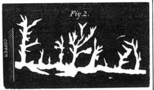
copper and nitrate of silver. The crystals of silver thus pro duced differ both in color and form, according to the strength of the solution. If it be very weak-say one per cent-the copper is fringed with black bushes of the metal, which, in growing, change their color to white without any alteration of crystalline form that can be detected by a powerful mi-
