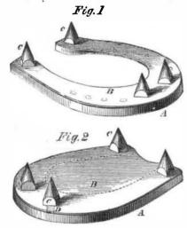
The annexed engravings illustrate an invention in which two important objects are aimed at, and, for ought we see, practically attained; one is the obviating of the very serious difficulty from the balling of the feet in snowy roads, and the other is a great facility in sharpening the corks in icy times, when the horse shoer is most hurried.
