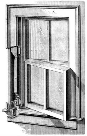
Now if either sash is to be taken out the cam-latch is turned part round, which permits the movable piece of the slide to be dropped into the recess, E, when the piece can be withdrawn, leaving a wide, open space sufficiently deep to release the
