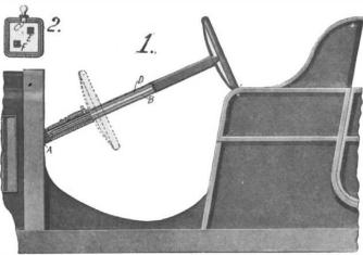
TELESCOPING STEERING GEAR FOR AUTOMOBILES.
