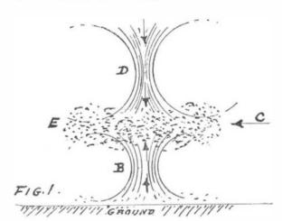
The drops of rain in a cloud being separated by air acting as a dielectric, electrify each other by influence; the resulting influence at the center of the cloud being an enormous electrostatic strain, which is relieved by lightning.
