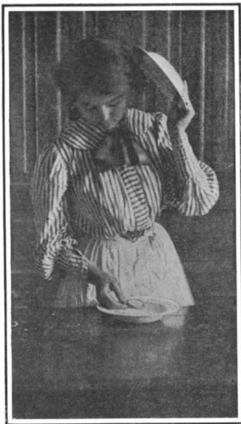
Soup plates as sound reflectors.
