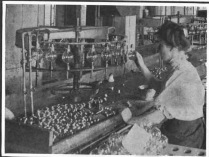
Placing the threaded brass collars on the necks of the bulbs.
