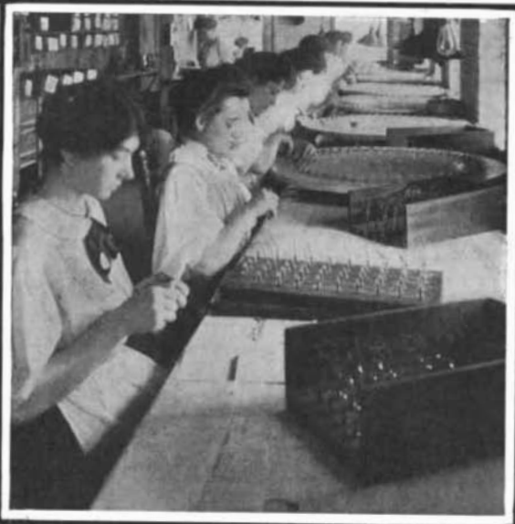
Pasting and straightening tables—straightening in the foreground.
