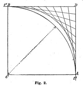
tained differs (in the case of the middle radius by as much as 4 per cent) from a true circle is seen in Fig. 2. As a matter of fact, both in this case and in the former more general case, the envelope obtained is a parabola touching DA, DB at the points  $t_1$  and  $t_2$ .
