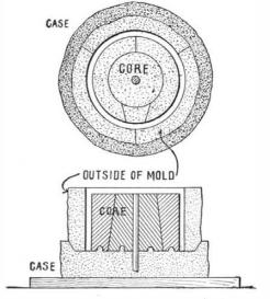
Fig. 22.—PLASTER MOLD READY TO RECEIVE CEMENT MIXTURE.
