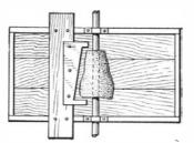
Fig. 18.-TEMPLATE FOR INNER PART OF CORE.
