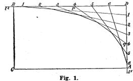
Let CA, CB be the axes of the required ellipse. Complete the rectangle A CBD, divide DA and DB each into 13 equal parts, and draw lines as shown, each of which will thus be a tangent to the required ellipse.
