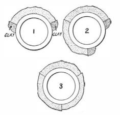
Fig. 15.—SUCCESSIVE STEPS IN MAKING THE OUTSIDE MOLD.
