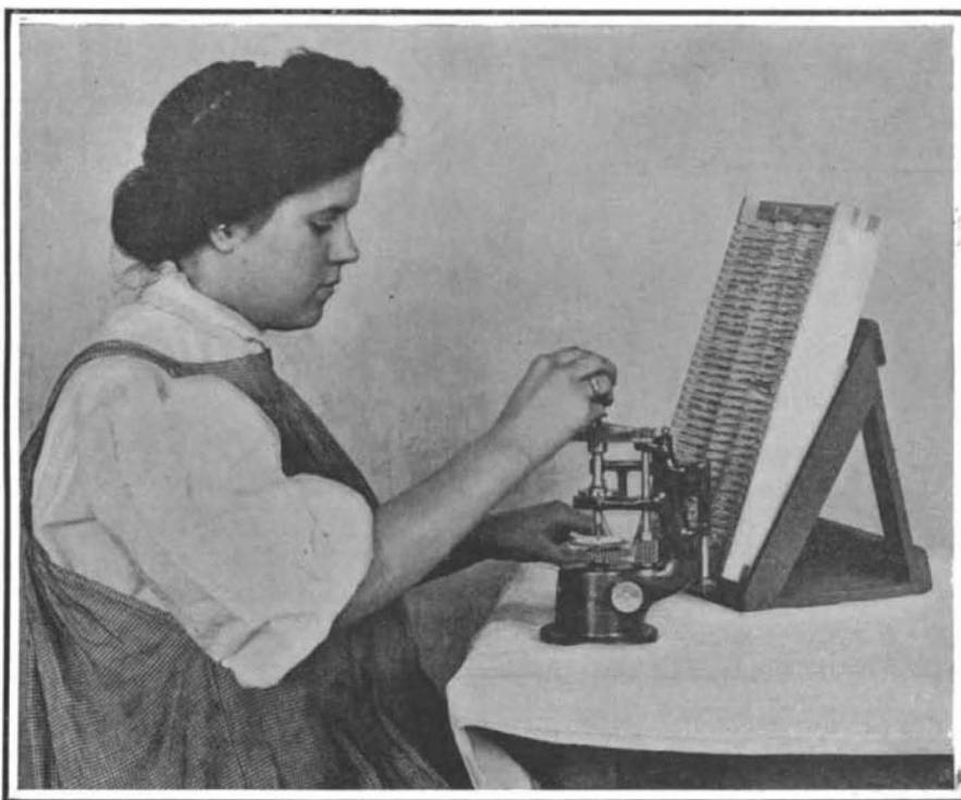
Making the oval cut with a diamond point on an oval swinging upright lathe.
