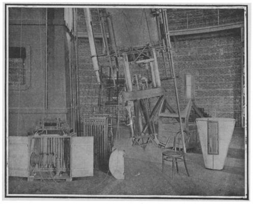
Bruce spectrograph fitted to the Yerkes telescope.
