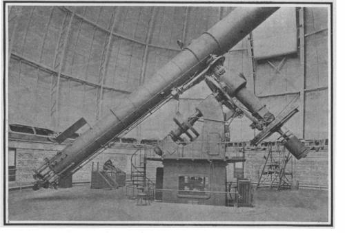
The Yerkes telescope with floor raised to highest position.
