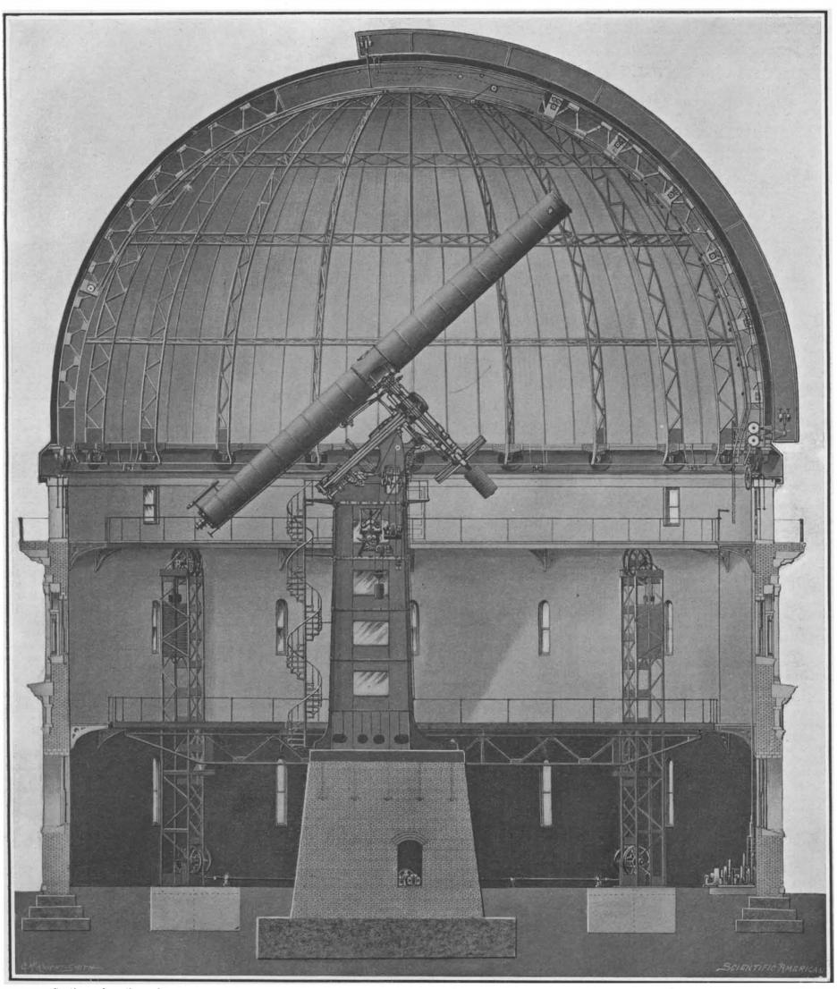
Section taken through the 90-foot dome of the Yerkes Observatory, showing the mounting of the 40-inch telescope and the 75-foot elevating floor.
