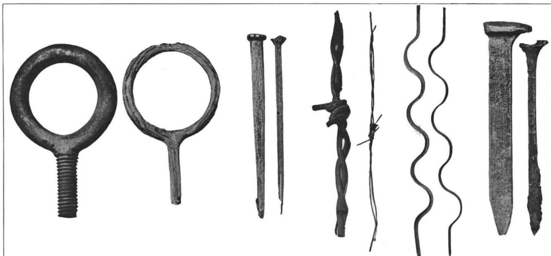
Ingot iron. Loss, 15.5%.
