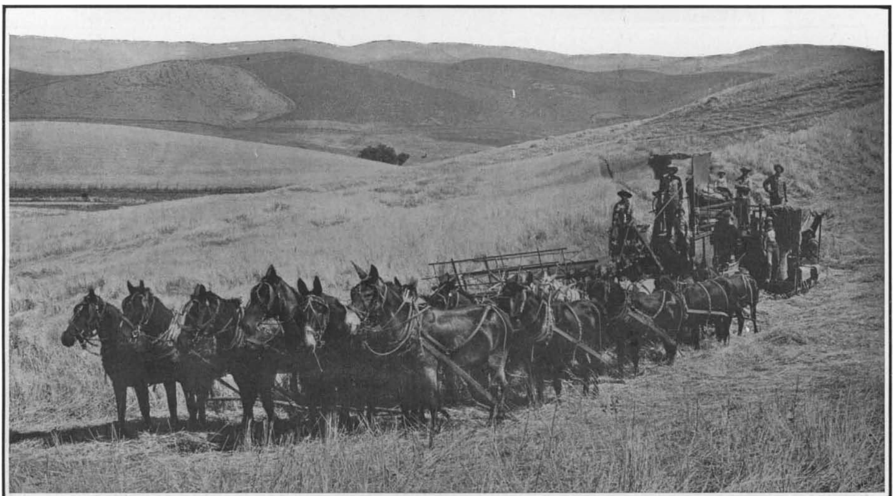
A COMBINED REAPER AND THRESHER DRAWN BY THIRTY HORSES AND MULES AT WORK ON A FIELD OF BARLEY IN OREGON.
