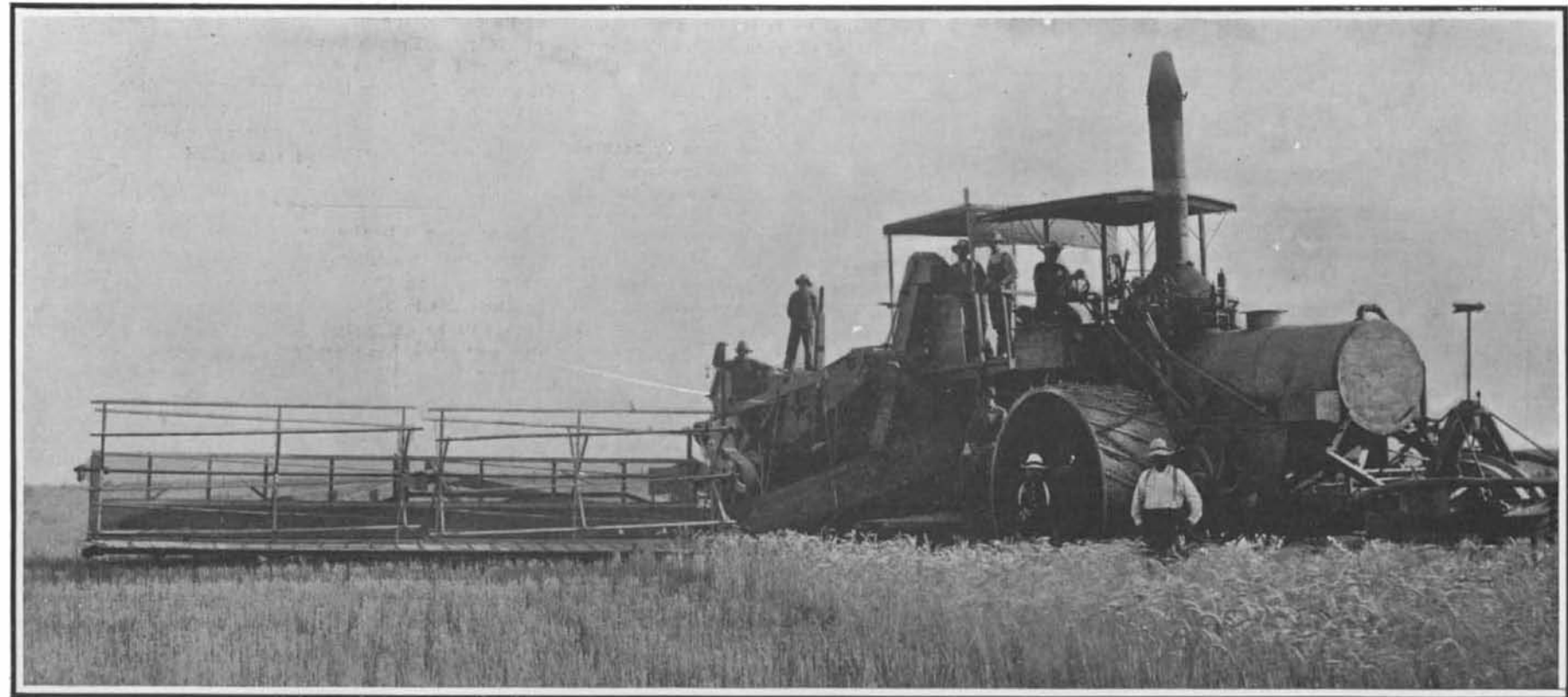
The harvester is shown at work in the wheat field of an Idaho corporation that owns 10,000 acres. The average yield on this ranch is 30 bushels to the acre. FRONT VIEW OF THE HARVESTER COMBINE SHOWN ABOVE.
