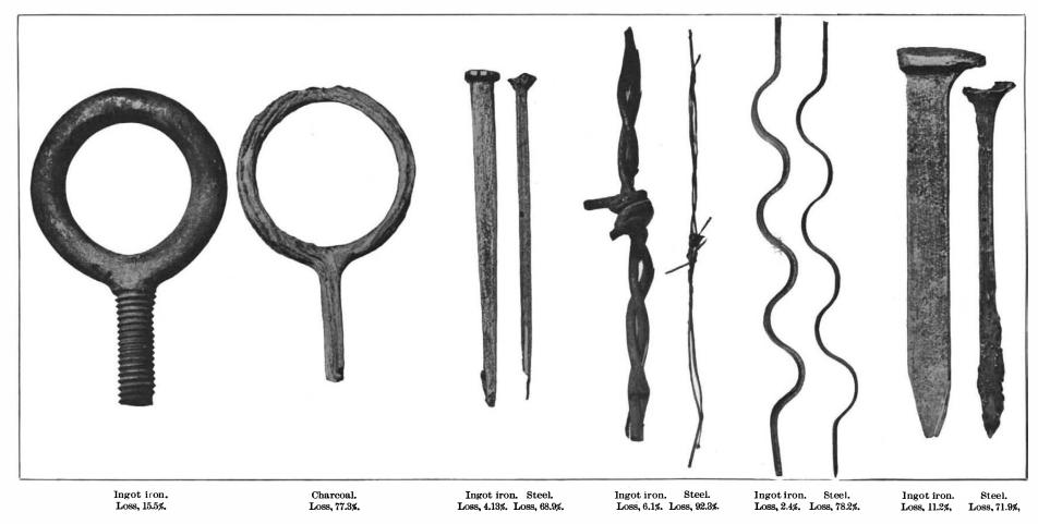
CORROSION TESTS IN BATH OF 25 PER CENT SULPHURIC ACID.
