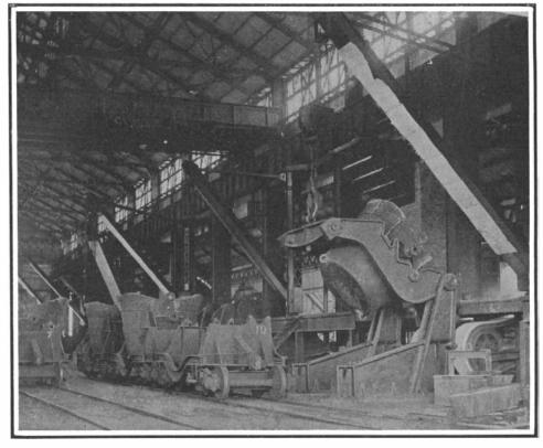
The molten iron trom the turnaces is brought to the open hearth furnaces in 60-ton ladles, one of which is here shown.
