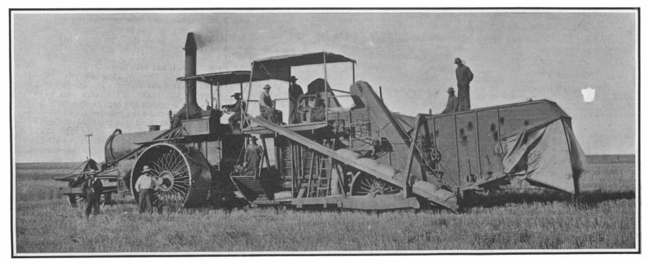
This machine cuts the wheat, threshes it, and delivers it ready sacked in one continuous operation. REAR VIEW OF A 50-HORSE-POWER HARVESTER COMBINE.
