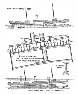
In the two diagrams of the "Yankce" the portions of the ship from which the water was expelled are shown in white.
