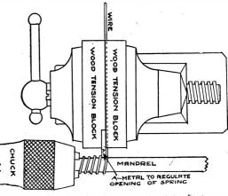
METHOD OF WINDING AN OPEN SPRING,
