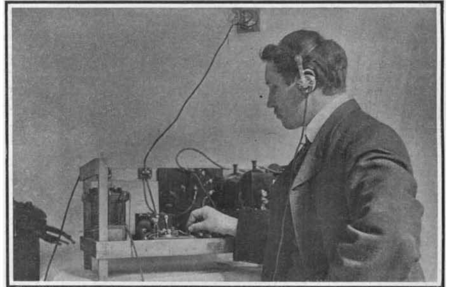
The wireless set employed by the Signal Corps for aeronautic use. The total weight is about 70 lbs. An 8-volt, 20-lb. accumulator supplies the current.
