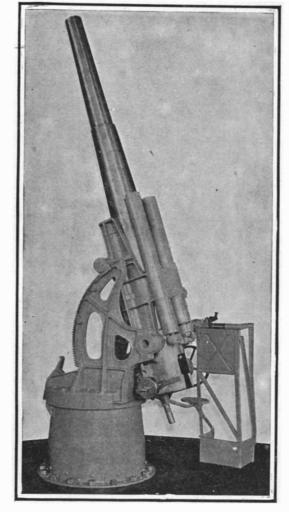
The 4.2-inch Krupp gun for aeronautic attack, on a naval mount.
