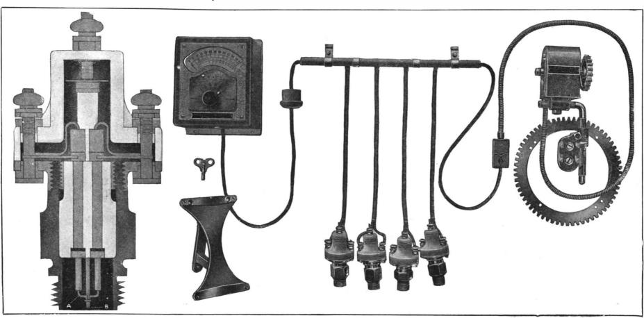
Spark plug fitted with thermo-couple.
