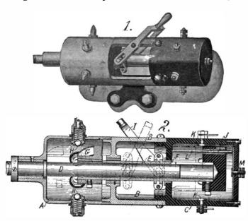
COMBINED TIMER AND DISTRIBUTER FOR INTERNAL-COMBUSTION ENGINES.
