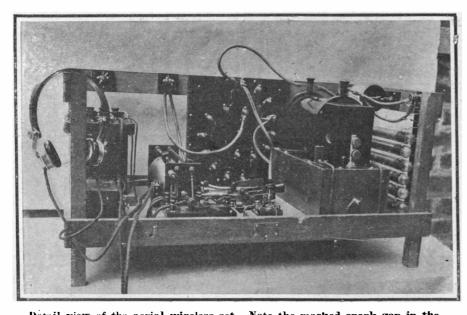
Detail view of the aerial wireless set. Note the masked spark gap in the upper right-hand corner of the frame.
