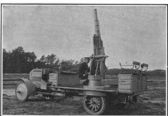
The 3-inch 12-pounder Krupp field piece for airship attack. The weapon can be brought to a maximum elevation of 75 degrees. The motor car on which it is mounted is of 50 horse-power and has an average speed of 30 miles an hour.
