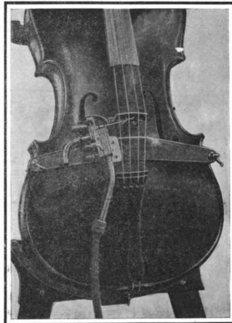
Fig. 2.—View of the instrument, showing mounting of the valve mechanism and aluminium connection between the bridge of the instrument and the valve.
