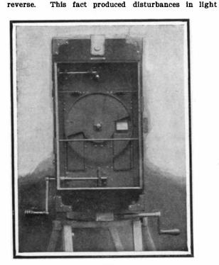
Fig. 1.—The face of the camera with lenses removed.
