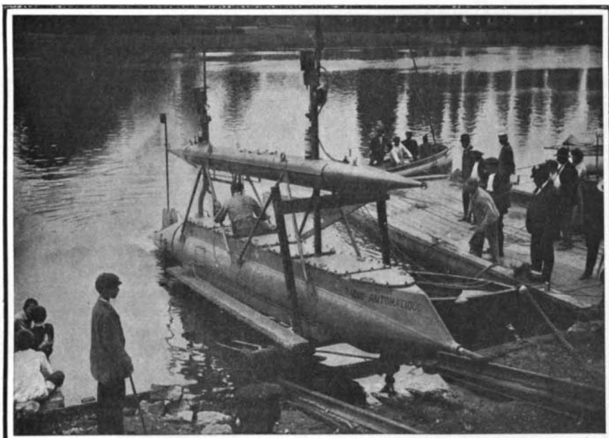
Launching the improved Gabet wirelessly-controlled torpedo.
