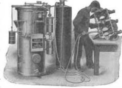
Torch is invaluable for cutting steel piling and structural iron, and for wrecking steel and iron work.
