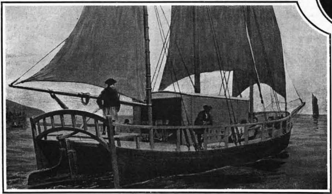
Fig. 3.—PATRICK MILLER'S DOUBLE-HULLED PADDLE BOAT DRIVEN BY MAN POWER. 1786.
