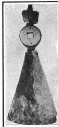
Round shank could be turned in the hub to change pitch.
