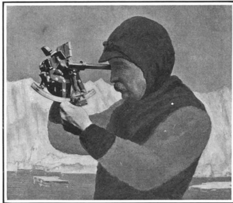
How the sextant is manipulated in measuring the sun's altitude.
