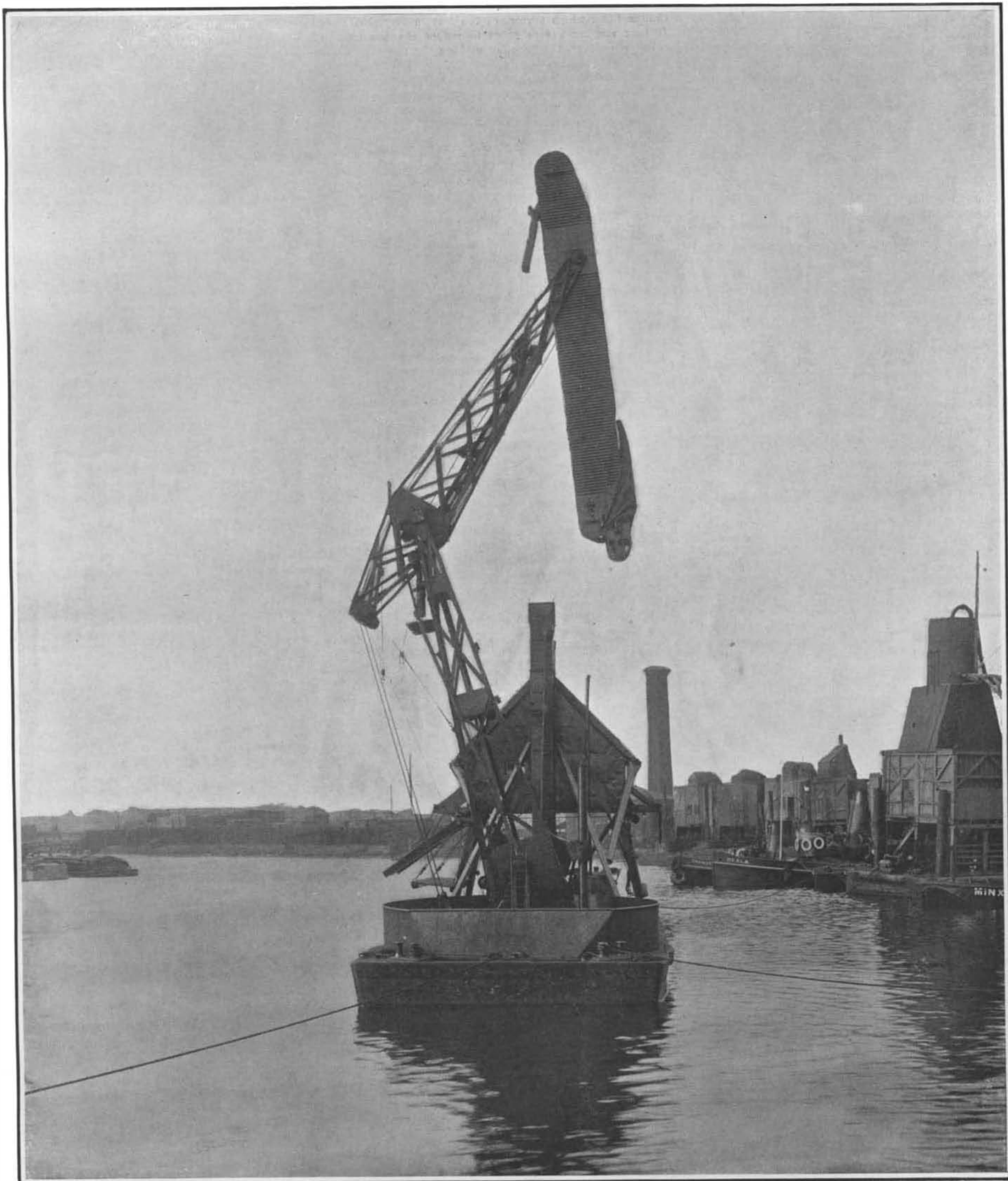
The illustration shows the height to which the elevator can be raised to go over the side of a ship.
