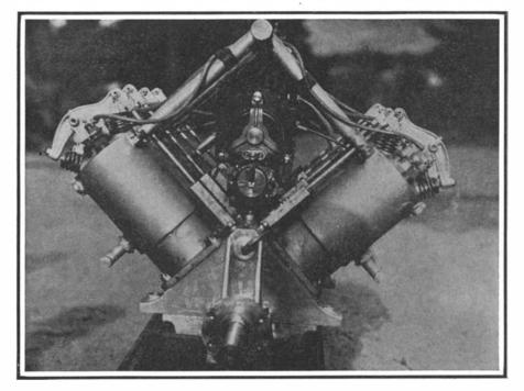
60-horse-power, 8-cylinder water-cooled motor of the winning
