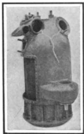
1. Monogram of the Scientific American and an attempt to "forge" the publisher's signature in half-inch boiler plate. 2. Aluminium automobile cylinder with crack repaired by oxy-acetylene welding.
