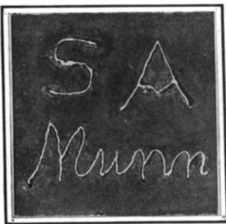
1. Monogram of the Scientific American and an attempt to "forge" the publisher's signature in half-inch boiler plate. 2. Aluminium automobile cylinder with crack repaired by oxy-acetylene welding.
