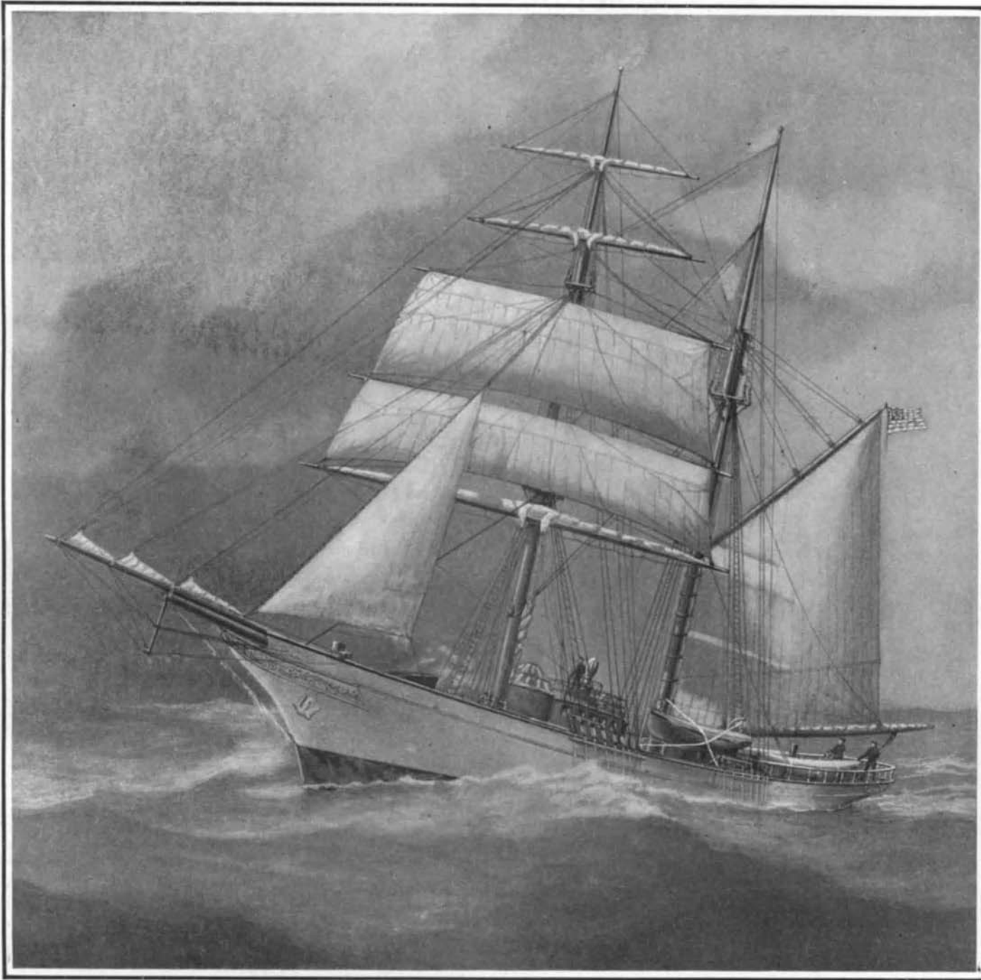
This interesting vessel is being built for the Carnegie Institution at Washington. Her survey of the oceans will form part of a comprehensive survey of the whole world, on land and sea, by which the magnetic variation of the compass is to be determined. No iron, steel, or other magnetic material will be used in her construction.
