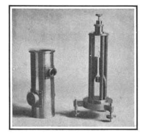
Féry photometer, with copper cylinder removed.
