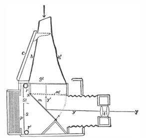
Fig. 8.—A reflecting camera shown in section with magazine plate holder attached.
