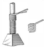
HOW TO WIND A SPACED COIL SPRING.
