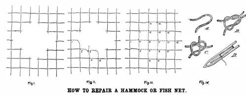
The knots are formed by pinching the meshes, as at 5, for instance, into a loop, as shown in Fig. 4 at A. Then threading the cord through the loop, a knot is made, either a flat or true lover's knot, as shown at B, or better still a fisherman's bend knot, as shown at C. The latter is not only easier to make, since it only passes through the eye once, but it will not slip so easily.
