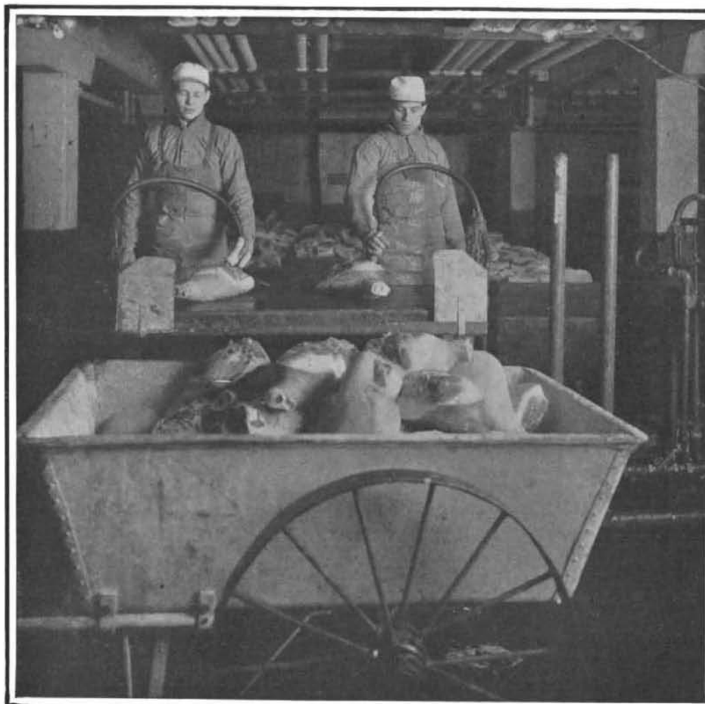
The solution of salt, sugar, and saltpeter is injected to the bone to insure that the impregnation of the meat shall be very thorough.
